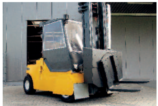
Rotator with sideshift for foundries and weighing system
