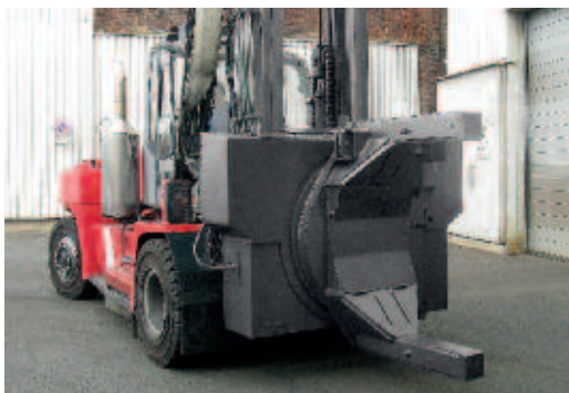
Rotator for foundries with full protection and converter handling arms
