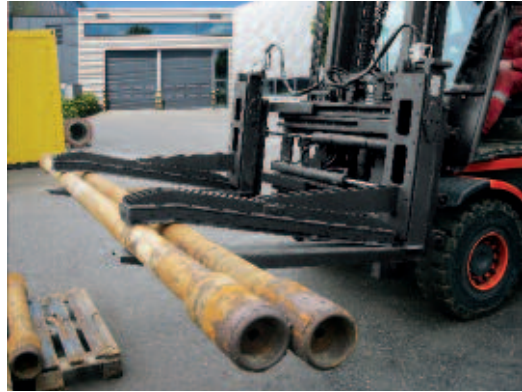
Fork positioner with load stabilizer
