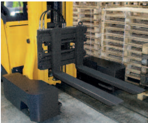
ZVKGS, narrow design for reach trucks
