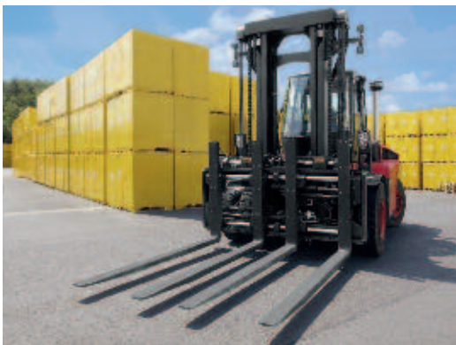
Special fork positioner with 4 forks
